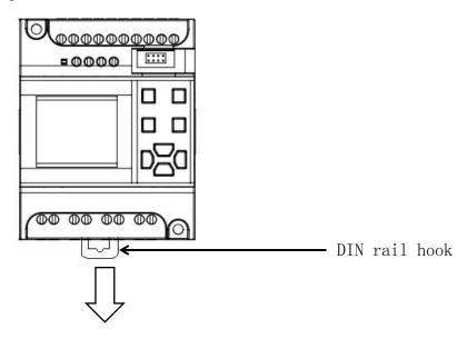
RTD temperature module can be mounted on 35mm DIN rail, When you remove, pls kindly simply pull the DIN rail's assembly hook, then the module could be removed.
