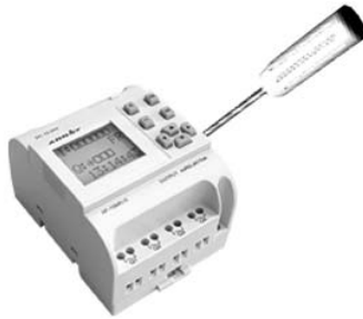
Fig. 2.2 Removing LCD panel as instructed
