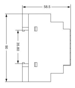
Installation Dimension of APB-12 Series (mm)
