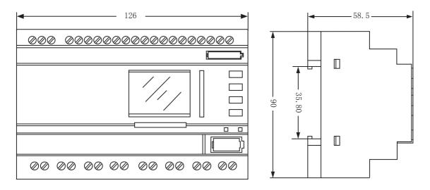
Installation Dimension of APB-22 Series (mm)
