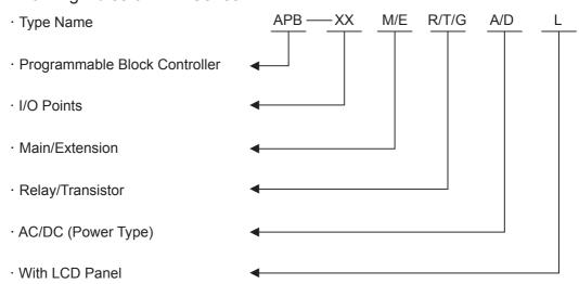
Note: M means main machine, E means extension module; R means relay output, T means NPN transistor output, G means PNP transistor output; A means AC type, D means DC type; C means real-time clock; The economical type is supplied without LCD panel, and the basic type is supplied with LCD panel.
