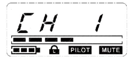
The display shows CH 1, in which 1 represents that the first channel is used currently.
